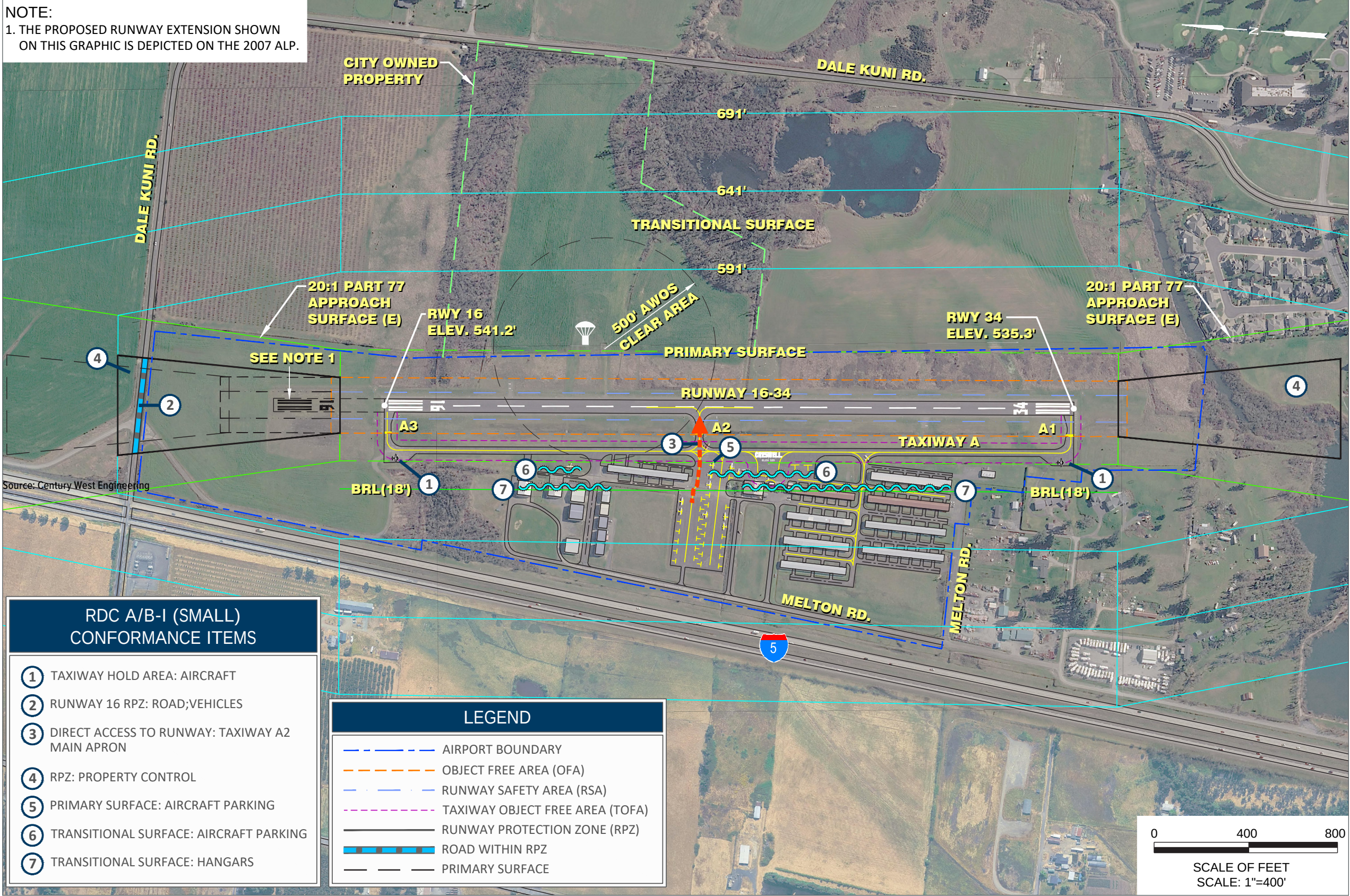
Figure 3-6 – Non-Conforming Conditions - Airside Facilities
